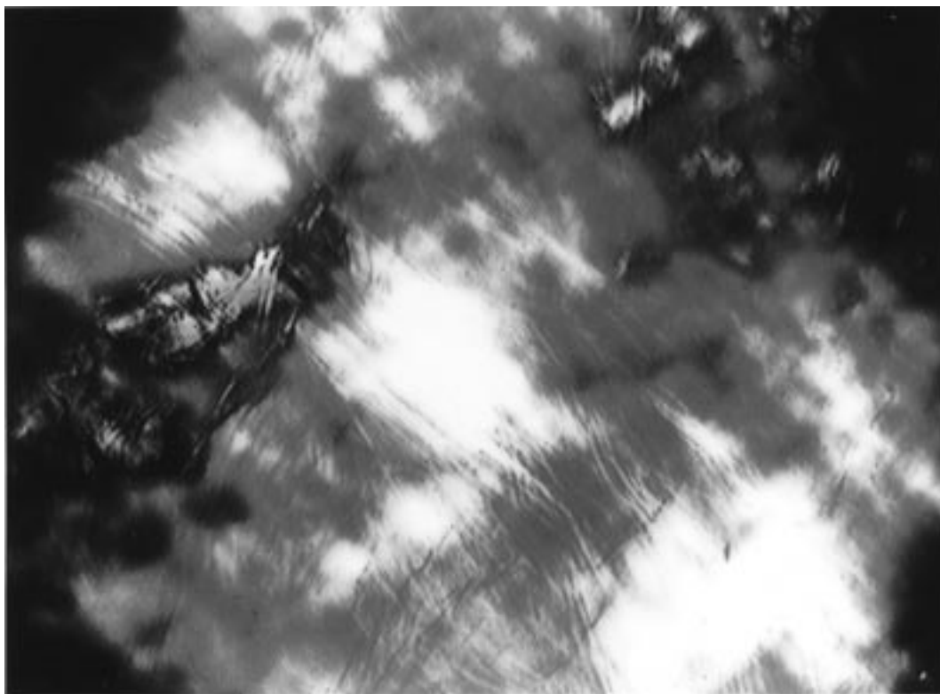
Figure 2. Microscopic picture of a gel prepared from 2a in chloroform. The gel was placed between crossed polarized filters.
